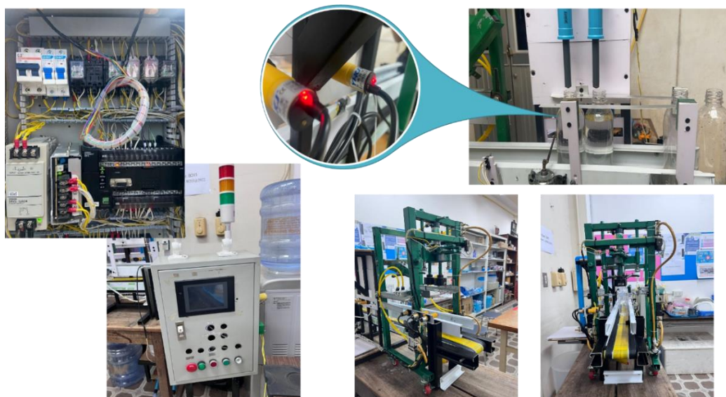
Figure 1. The integrated automated bottling system setup including PLC, HMI, and conveyor unit.
